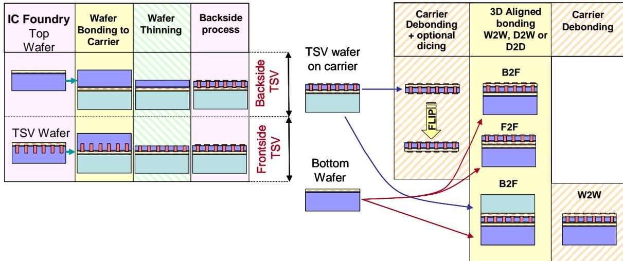
Figure INTC3 Schematic Representation of the Various Key Process Modules and 3D-stacking Options when using Through-Si-Via 3D-WLP Technologies<sup>4</sup>
