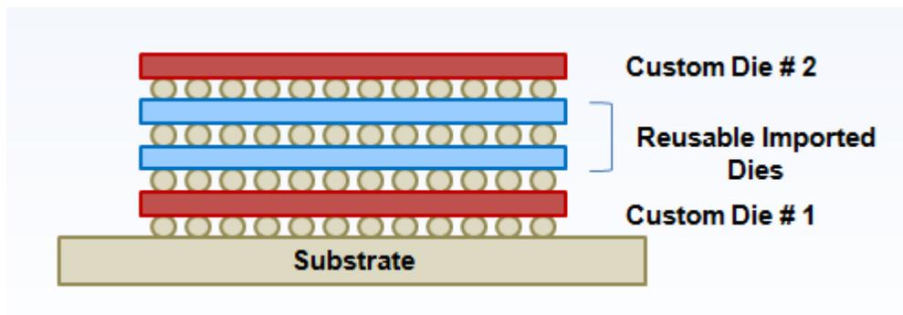
**3D Stack:** Integrating multiple heterogeneous die on top of each other in a conventional package
