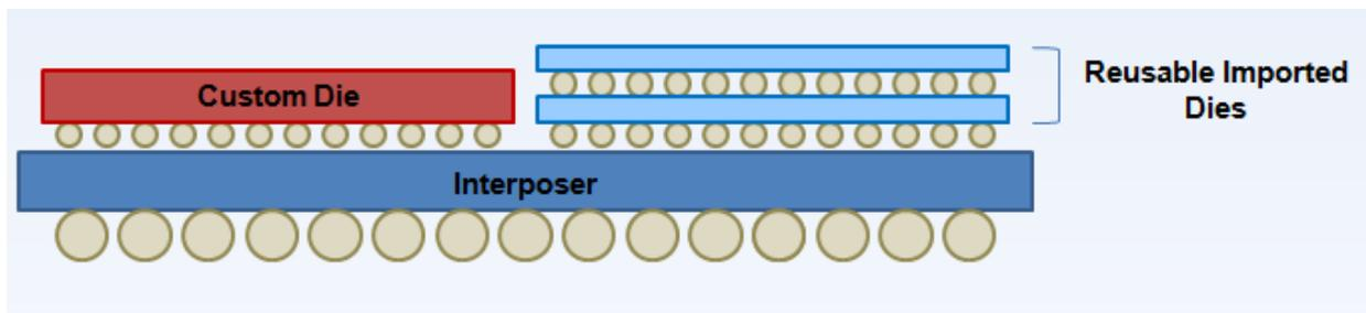
**2.5D Stack:** Integration of multiple die (and/or homogenous die stacks) side-by-side on silicon or glass interposer
