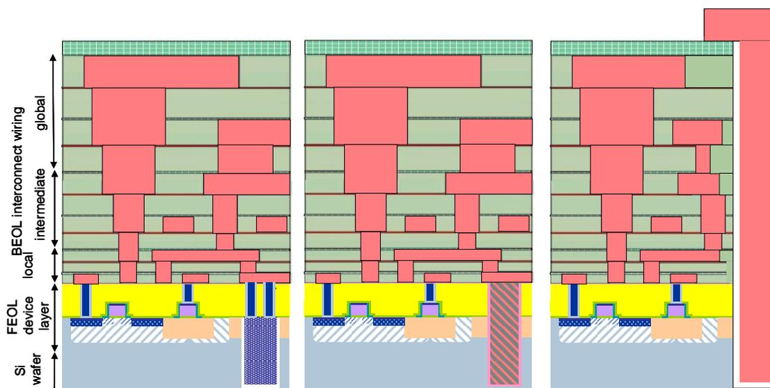
Figure INTC1 Schematic Representation of TSV First, Middle and Last Process Flows
