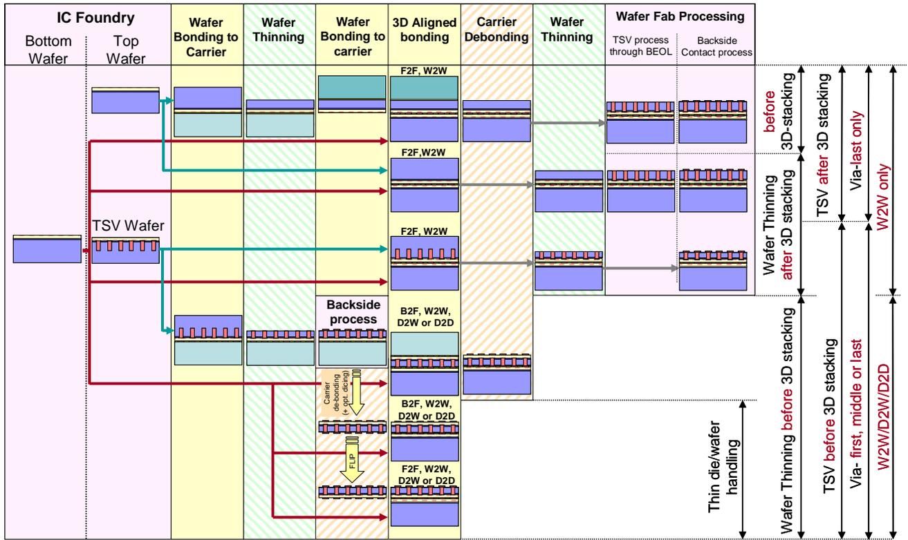
Figure INTC2 Schematic Representation of the Various Key Process Modules and 3D-stacking Options when using Through-Si-Via 3D-SIC Technologies<sup>3</sup>
